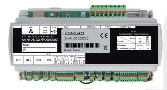
The pascom XS.net barrier module has been developed for controlling the barrier system and is connected to the pascom XS.reader via the RS232 / RS485 interface. The device is suitable for cap rail mounting.
