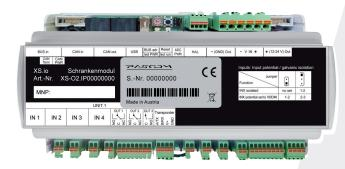
The pascom XS.io barrier module has been developed for controlling the barrier system and is connected to the pascom XS.reader via the RS232 / RS485 interface. The device is suitable for DIN rail mounting.
